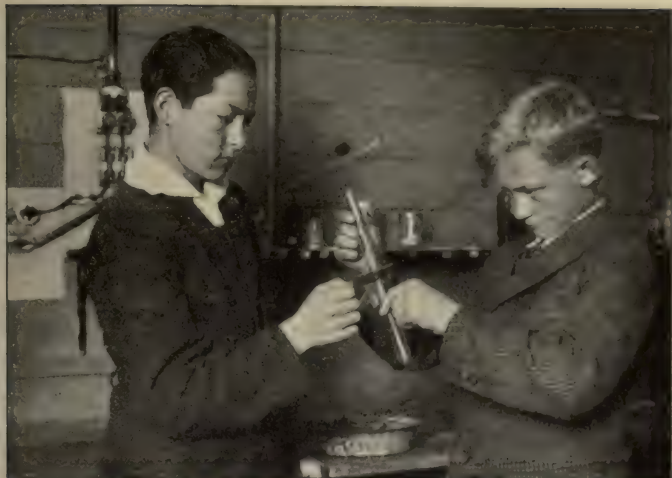
FIG. 150. The lower test tube is full of air; the upper, of gas. What will happen when the cardboard is withdrawn?
